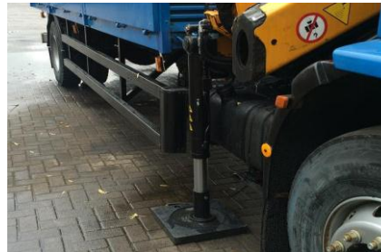
Leg deployed but beam not extended
