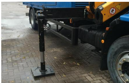
Beam only partially deployed
