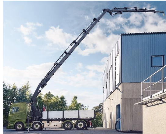
Figure 2: Lorry Loader Crane
